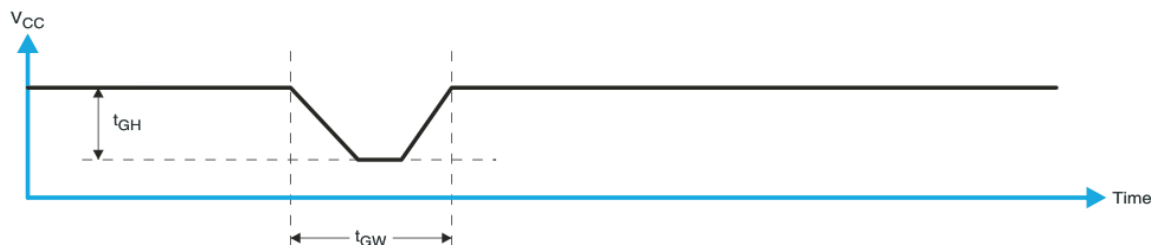
Figure 21. Glitch Width And Glitch Height
